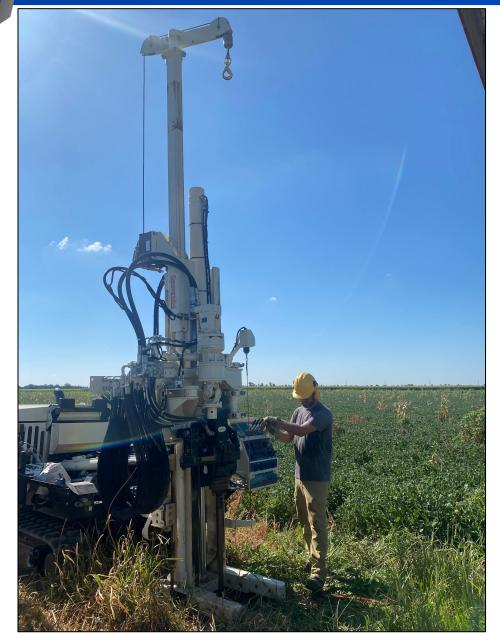
Electrical conductivity (EC) logging provides lithologic information about soil conductivity and resistivity
