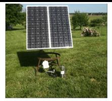
Sunpumps: (diaphragm pump, brass and stainless steel, with brushes, design for shallow well), (air filled motor cavity), (DC power only).
