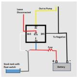
Figure 2. Wiring diagram for a float system.
