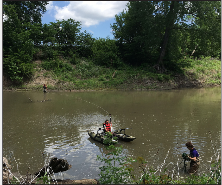
Tim Keane (across river, Co-PI), Trisha Moore (on boat, Co-PI) and Max Burden (undergrad assistant) surveying Cottonwood streambed bathymetry with total station. Photo courtesy Kari Bigham.
