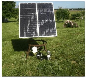
Figure 1. Solar pump demonstration unit.
